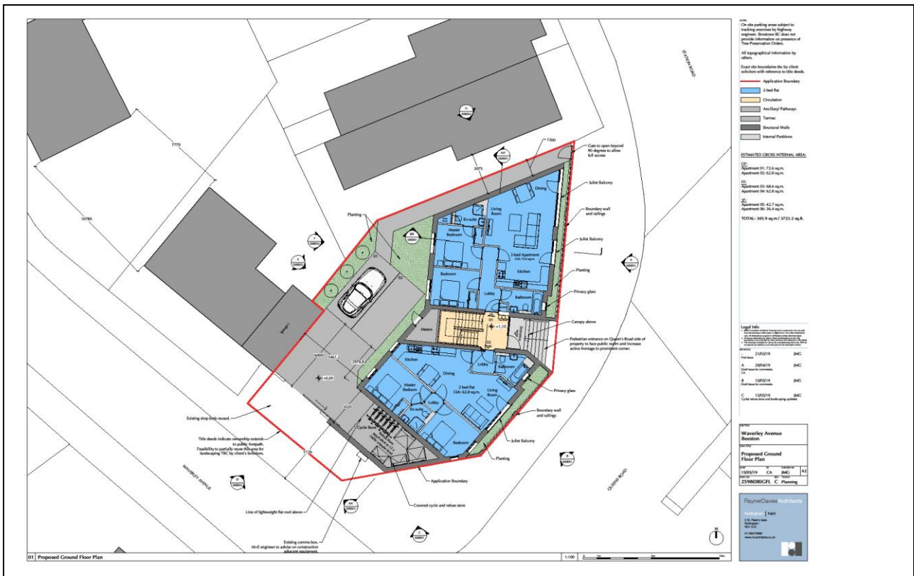
Proposed ground floor layout
